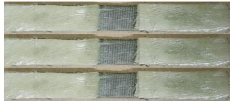
**Fig. 2** Compression Test Specimen
